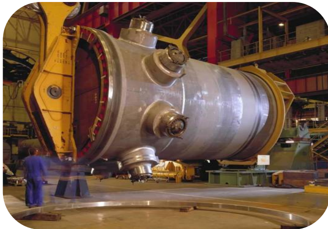
Reactor Pressure Vessel machining at AREVA Chalon St-Marcel Heavy Components Plant
